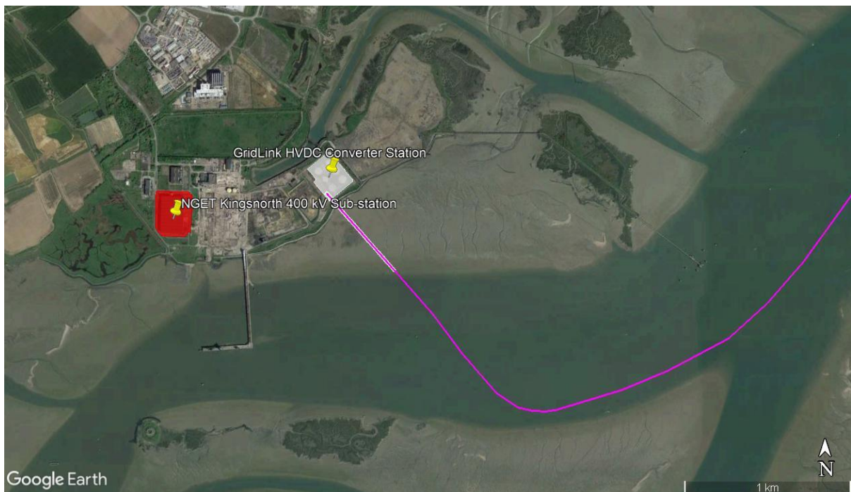
Figure 7 HVDC cable route, converter station site and National Grid Kingsnorth sub-station in UK
