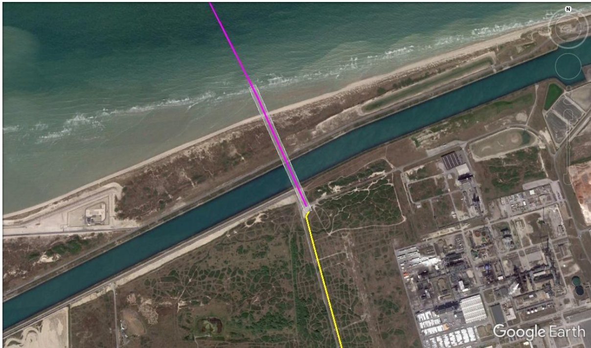
Figure 12 Horizontal Directional Drilling (HDD) at Dunkerque Shore Crossing
