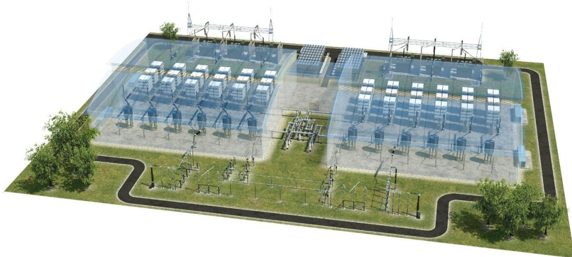
Figure 23 Example of converter station design (source: Siemens Aktiengesellschaft)
