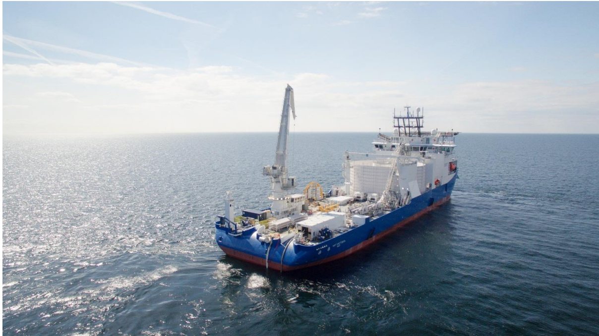
Figure 11 Typical Vessel used to lay the Subsea Cables (source: NKT)
